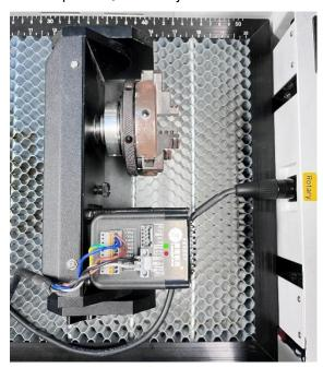
3. Connect the rotary axis attachment via the control cable with the connector of the motion system. The connector is located inside the right front of the laser. Connected it to this interface and fixed, and then you have finished the device connection. Like below:
