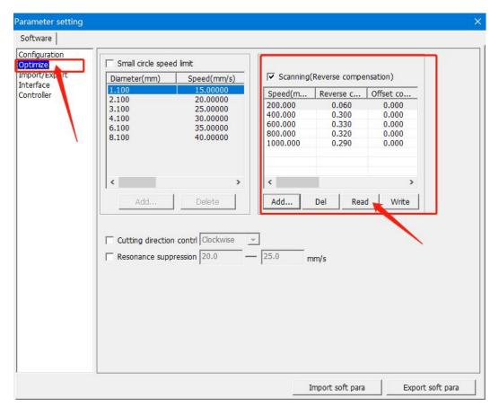
The particular values are showing with a picture in folder of laser software on the USB flash drive and on the Anodized aluminum piece that came with your machine.
