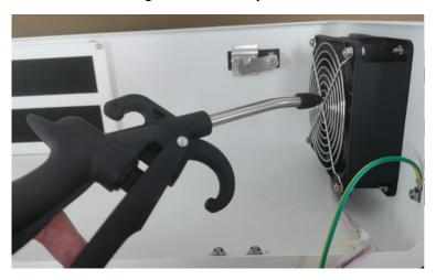
3. Remove the screws which fixed the cooling fan, take out the fan, and use an air blow gun or a pump to blow the dust away.
