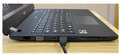
One USB cable can control the communication between the computer and the dsp and the camera at the same time.
