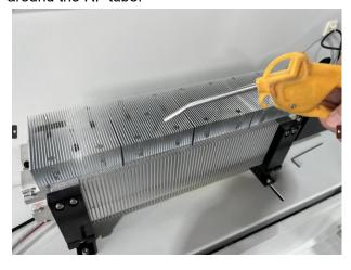
5. After cleaning the dust, reinstall the fan on the RF tube and the cleaning is finished.
