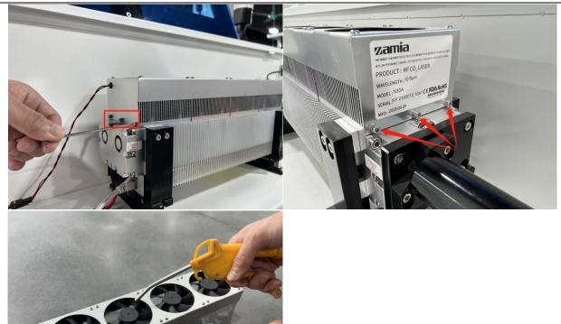
4. Use an air blow gun to blow away the dust on the RF tube, then you can use a rag to wipe the dust around the RF tube.
